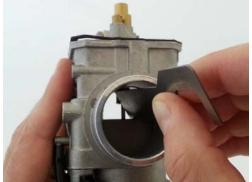
d) The position of the cap of the carburetor must be fixed by means of the fixation plate (pos. 1 see illustration below, ROTAX part no. 251 790, see attached picture).
