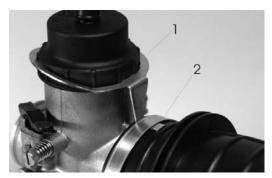
f) Only one rubber gasket is allowed to be used in the carburetor cap.
