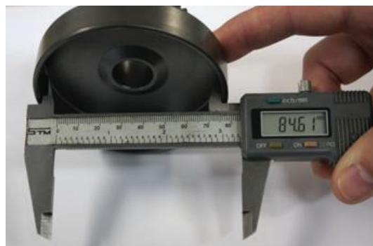
The inner diameter has to be measured with a sliding caliper. The measurement has to be done in the middle of the clutch drum (in the contact area of the clutch drum).
