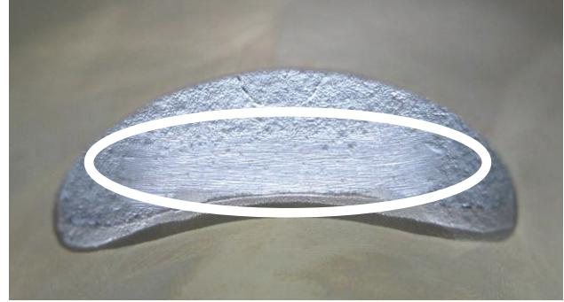
The exhaust port may show partial manual grinding done by the manufacturer to eliminate minor casting defects and to eliminate the NIKASIL burr at the end of the NIKASIL plating.
