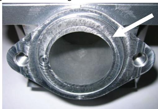
The top edge of the exhaust port may show either just a cast finish surface...
