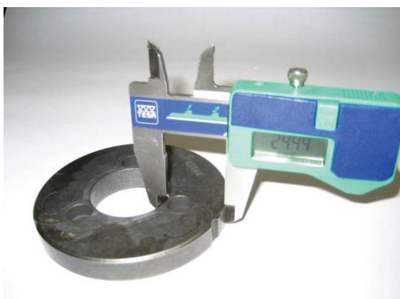
Measurement has to be done at the 3 open ends of the clutch shoes, 5 - 10 mm from the machined groove (all clutch shoes must be completely closed at measurement - no gap). No measurement may be below 24,10 mm.
