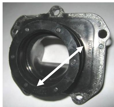
b) Some factory flash removal may be present at the conjunction of the inside contour and the carburetor stop mounting face. This is a manual trimming operation consisting of a small corner break of less than 3 mm in width. No additional grinding or machining is permitted.
