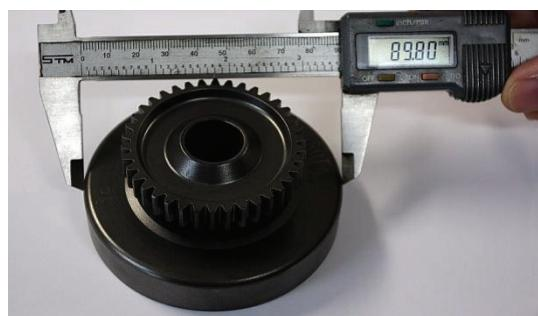
Diameter has to be measured with a sliding caliper just beside the radius from the shoulder (not at the open end of the clutch drum).
