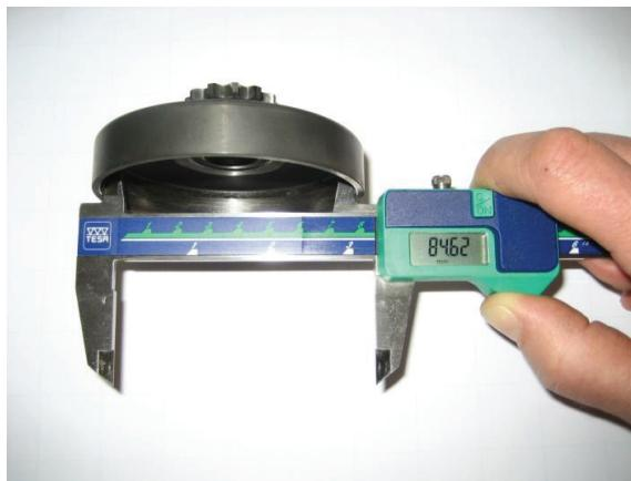
The inner diameter has to be measured with a sliding caliper. The measurement has to be done in the middle of the clutch drum (in the contact area of the clutch drum).
