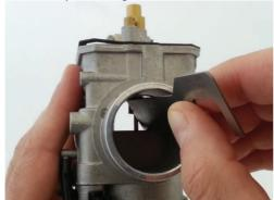
d) The position of the cap of the carburetor must be fixed by means of the fixation plate (pos. 1 see illustration below, ROTAX part no. 251 790, see attached picture).
