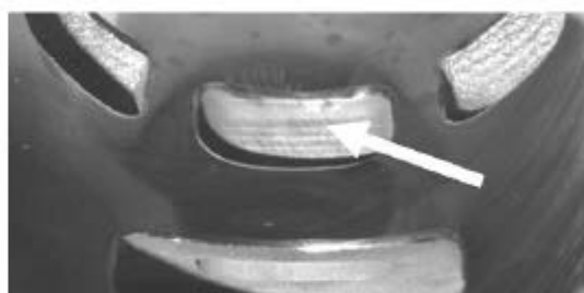
Single Core Cylinder: linear structured cast finish surface
